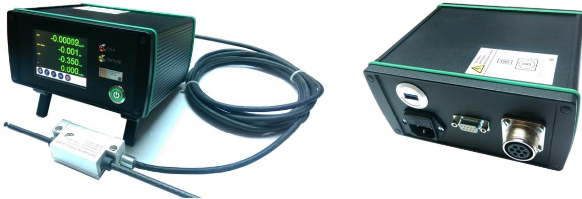
**The strain gauge full bridge** input channel has a high common mode rejection ratio (CMRR). The low-noise 24-bit sigma-delta ( $\Sigma$ - $\Delta$ ) AD converter, with low offset and gain drift (5nV/°C, 1ppm/°C), is synchronised by a frequency-stable clock ( $\pm 0.2\%$ ), with low frequency tolerance ( $\pm 0.1\%$ )
